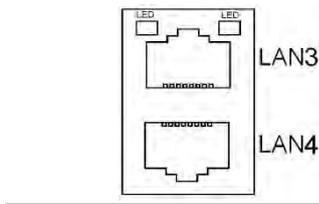
**LAN LED:** There's no light will on while using 10/100M LAN. The green light will on while using Gbe LAN
