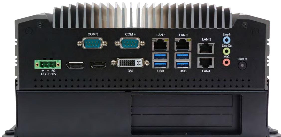
**Figure 1.4: Front view of EW420 with 2xPCIe x 1 slot**
