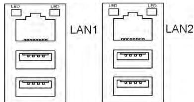
**LAN LED:** There's no light will on while using 10/100M LAN. The green light will on while using Gbe LAN
